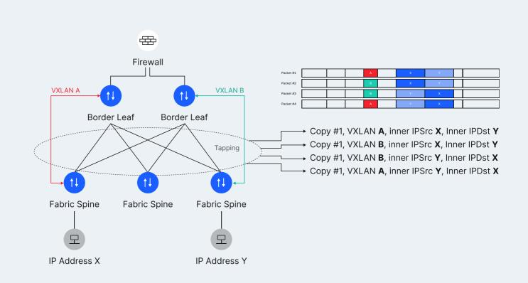
Traffic between IP X and IP Y passes the tapping two times and thus the same packets are visible twice at the tapping output. From user perspective every packet is received twice.
