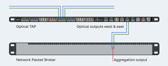
By utilizing the various filtering capabilities of the EXA48200 the user is able to further reduce traffic volume that needs to be processed, thus enabling quicker and more accurate analysis and troubleshooting. Moreover, incoming traffic can be VLAN tagged per physical port to allow easy identification at which physical port a packet original arrived.
