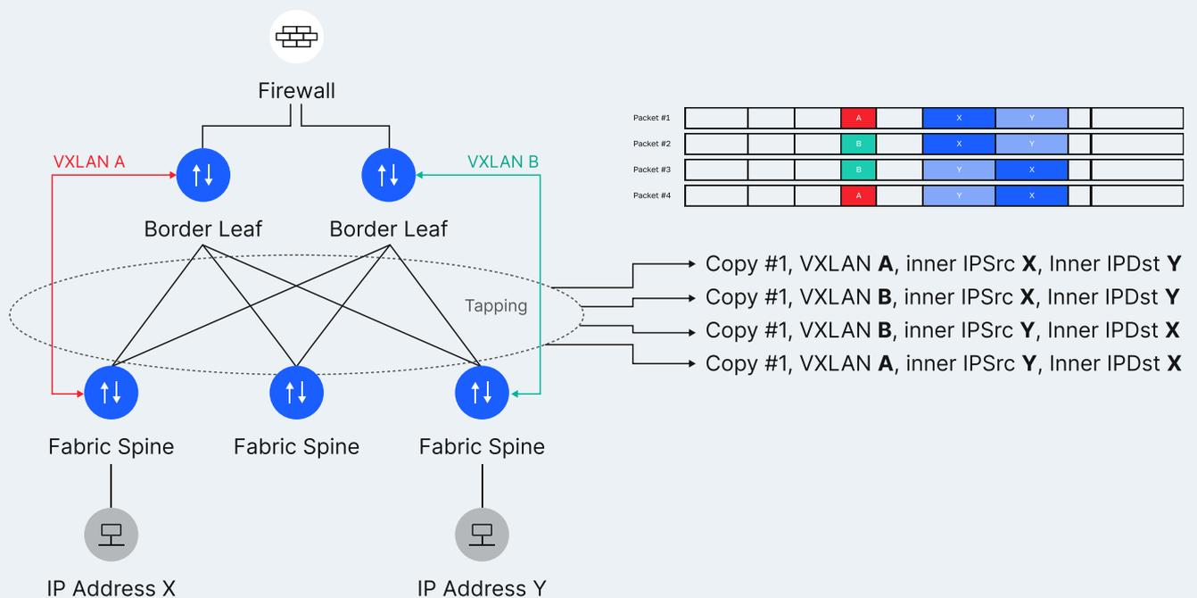
Traffic between IP X and IP Y passes the tapping two times and thus the same packets are visible twice at the tapping output. From user perspective every packet is received twice.
